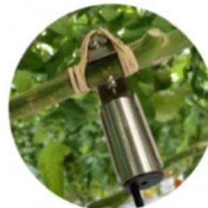
Sensor diameter variation Measures the diameter variations up to <math>\pm 1\mu\text{m}</math>
