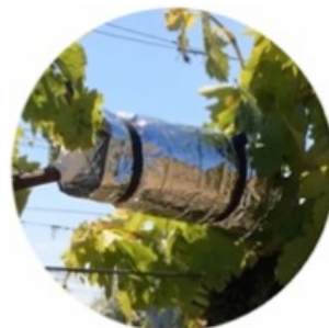
Sapflow sensor Measure the sapflow rate in g/h
